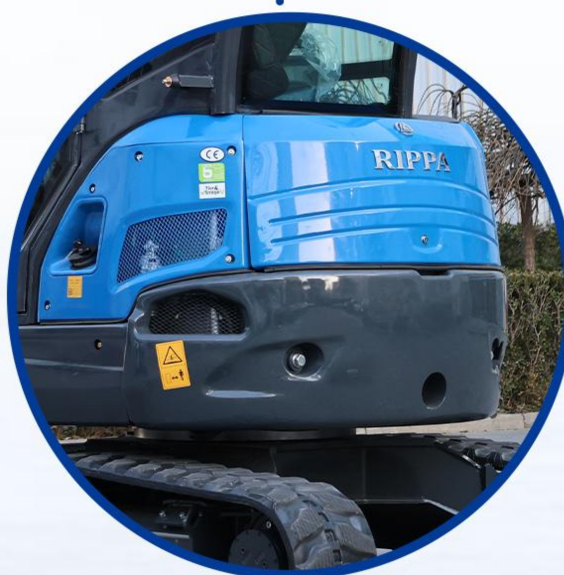
Counterweight-Real weight : 3.2Ton
