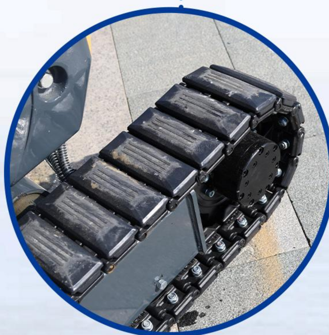
Steel tracks + rubber blocks for durability and ground protection
