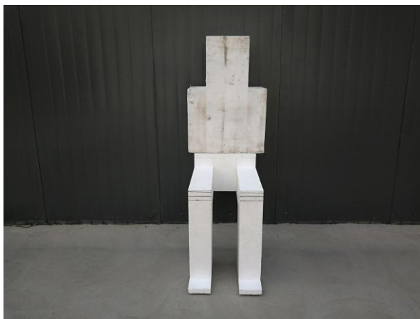
Figure D1 Deflection-limiting Volume
