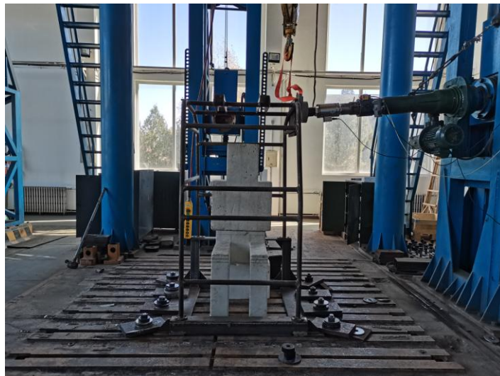
Figure. F1 Before the lateral loading test
