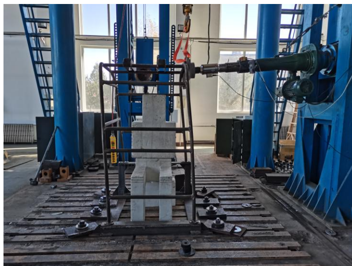
Figure. F2 After the lateral loading test
