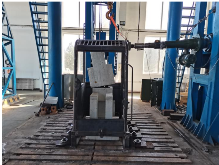
Figure. F1 Before the lateral loading test
