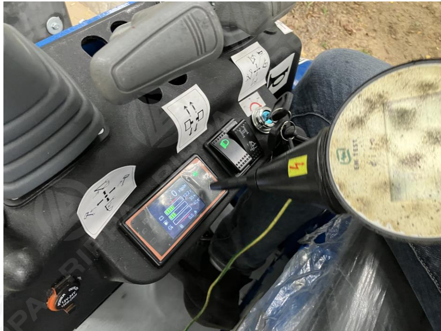
Photograph 2: Set-up for immunity test of ESD
