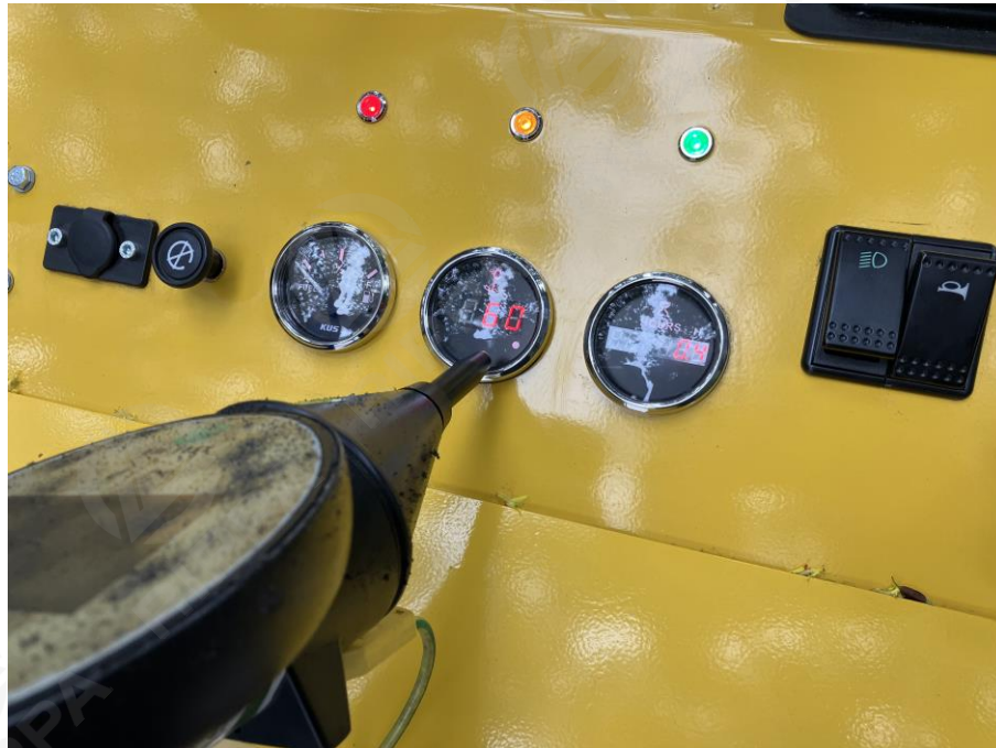
Photograph 2: Set-up for immunity test of ESD
