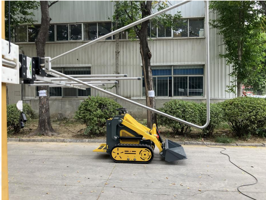
Photograph 1: Set-up for radiated electromagnetic disturbances above 30MHz
