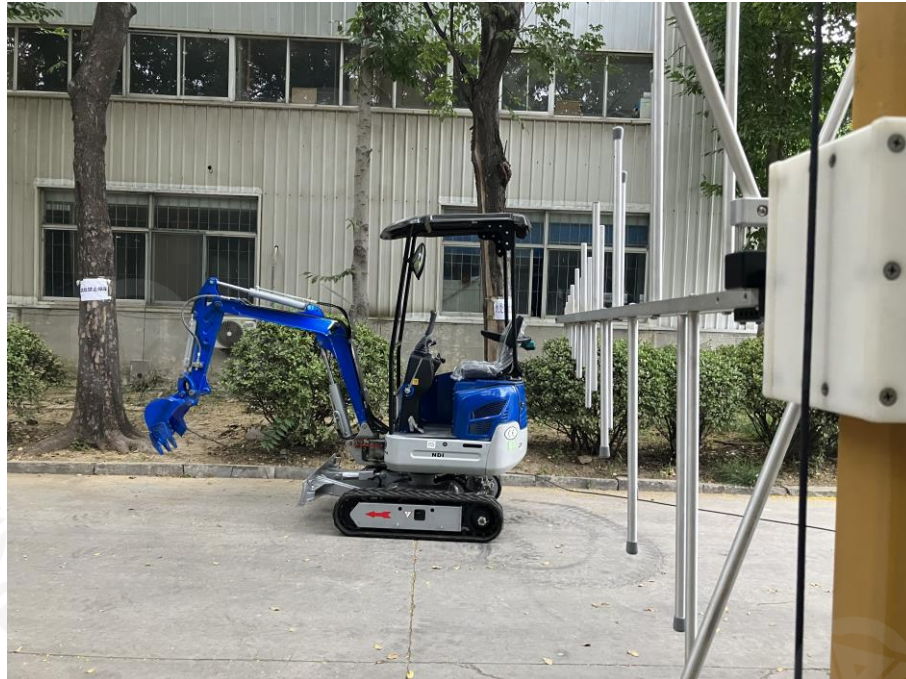
Photograph 1: Set-up for radiated electromagnetic disturbances above 30MHz
